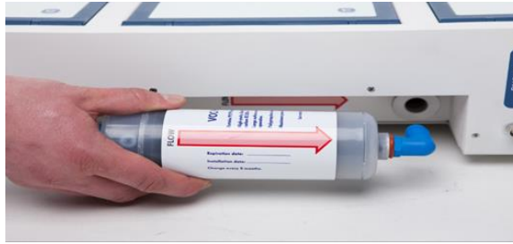
Figure 12.2 The way of pulling filter
