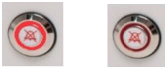
Figure 15.1 Alarm key which indicate the alarm condition
