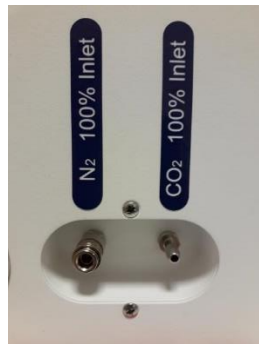
Figure 11.1 Gas inlets on the back of Mini MIRI® Dry and MIRI® Humidity multiroom IVF incubators
